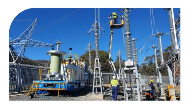
The 720kV AC test truck enables insulation testing of switchyard primary equipment of system voltages up to nominally 500 kV. This is achieved through the combination of resonant and conventional AC test equipment, assembled into a versatile mobile test system, which often removes the need for additional test trucks, resulting in a saving in testing effort and cost.
